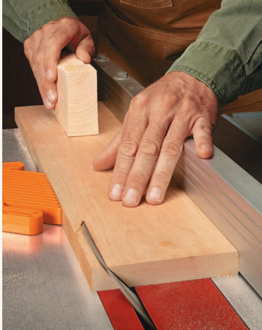
bevel cuts, there are a few things to mention. First, you'll get less cutting resistance and safer, cleaner cuts by starting with a sharp blade. I like to use a good quality rip blade. But a combination blade works almost as well.
